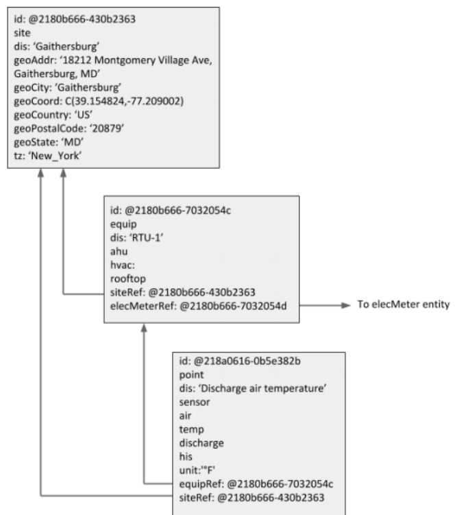
Figure 3 Example of Project Haystack ontology containing a site, equip and point entity. Source: Project Haystack; Reference Implementation – Applying Haystack Tagging for a Sample Building. On: https://marketing.project-haystack.org/images/white-papers/Reference-Implementation--Applying-Haystack-Tagging-for-a-Sample-Building.pdf ; accessed on 11-5-2021.
